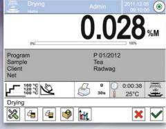
The main display features quick access bar providing instant access to basic settings and parameters of drying process.
